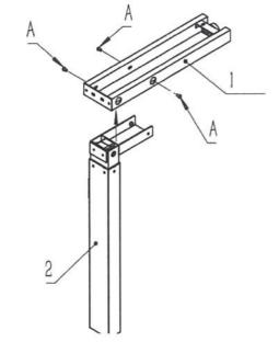
2.Fixing the bottom with the Allen key.
